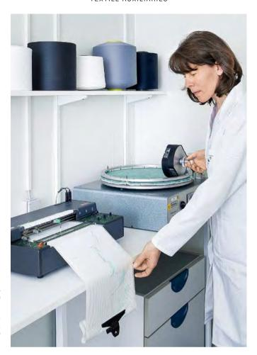
We produce a large number of auxiliaries for applying functional finishes to carpets. They are preceded by extensive testing, like measuring the effectiveness of our antistatic agents shown here.
