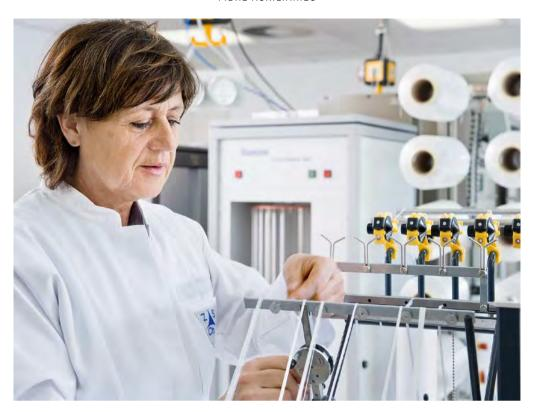
Our measuring technology enables us to determine various textile parameters that are important for the performance of our products. Here: preparing a yarn count measurement.
